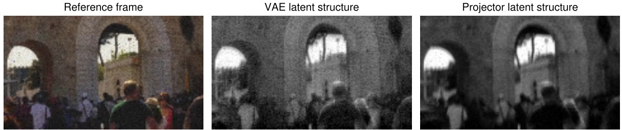
Fig. 5. Visualization of encoder-free latent projection. Given the same LQ input, we compare latents produced by a frozen VAE encoder and by the proposed pixel-unshuffle plus linear projector. Both latents share the same shape. We visualize their channel-invariant spatial structures using the first principal component (PC1). The projector preserves scene structures highly consistent with the VAE latent, indicating that it serves as a lightweight alternative for VSR inference.
